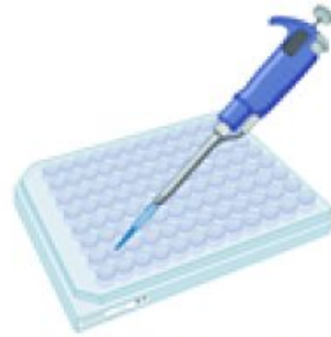
(B) Add 10 \mu l of a 10X concentrated solution of chemicals
